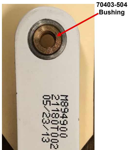
Figure 45-16 70403-504 Bushing Installed Into 21180-1 Lever
